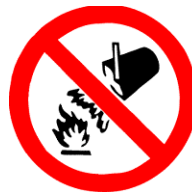
Water may not be used to extinguish fire
